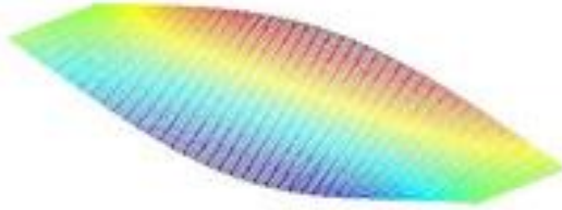
Mode 2: First Torsion Mode (6.78 Hz)
