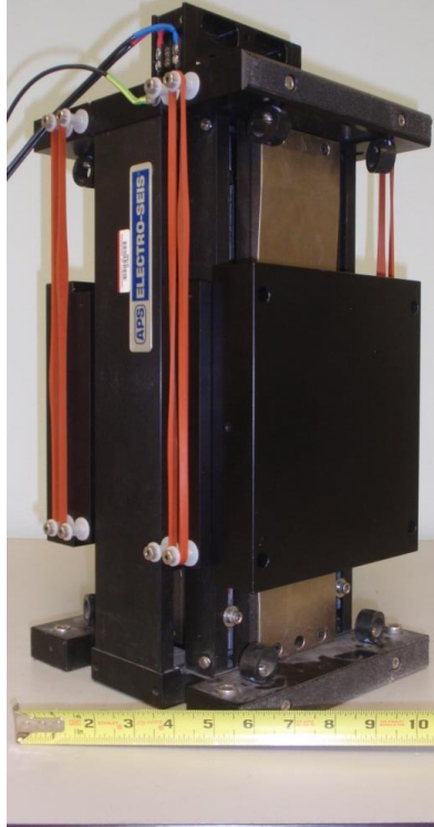
Figure 3.13 Electro-dynamic Shaker with Reaction Masses (Torres Goitia, AR, 2012).
