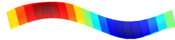
Mode 4: Second Bending Mode (21.7 Hz)
