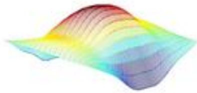
Mode 10: Deck First Bending Mode (34.7Hz)
