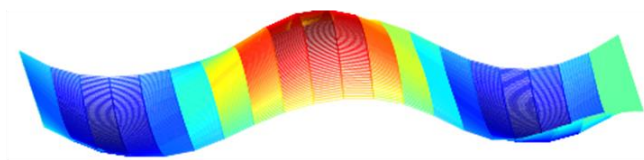
Mode 9: Third Bending Mode (40.4 Hz)
